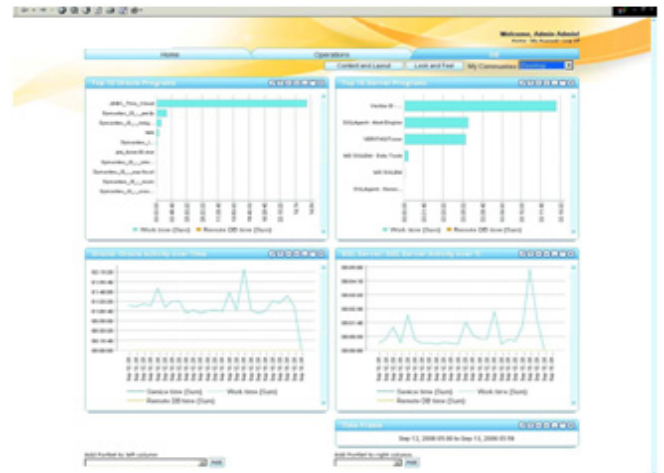
Figure 1 Using Application Service Dashboard, administrators can view performance data from heterogeneous database instances. For example, they can see top Oracle and SQL Server activities in the same display.
